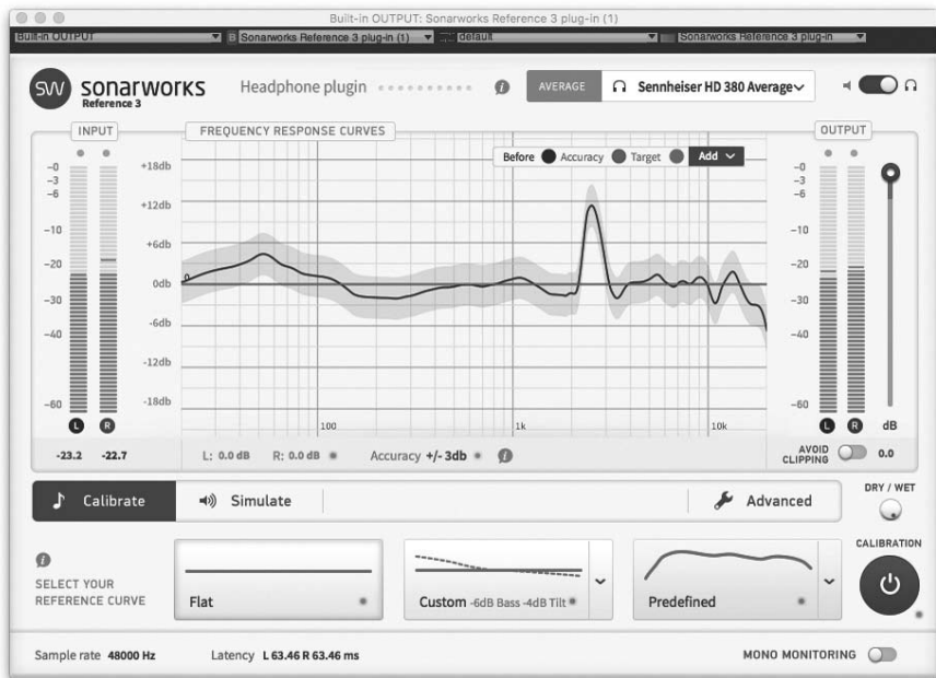
Figure 1. Software that compensates for inadequate frequency response of headphones. Screenshot by Author.
